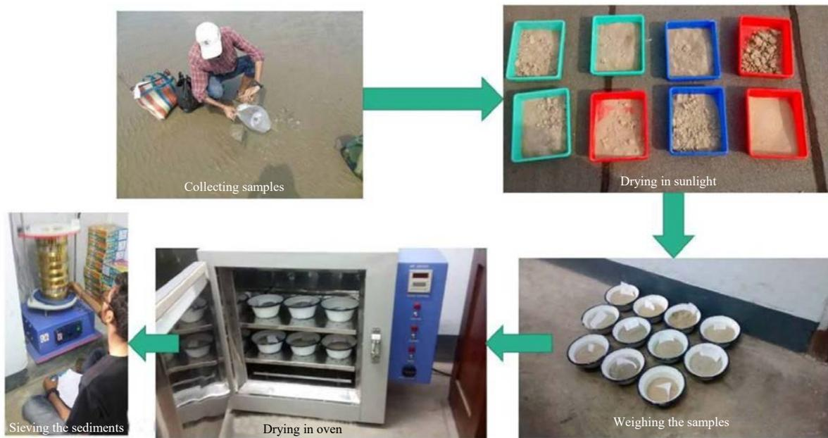
Fig. 3: Methodology of sample collection to preparation for grain size and sorting analysis
