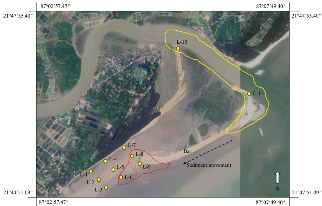
Fig. 7: Active estuarine sedimentation zone, marked by yellow, arrow indicates shore parallel sediment transfer from bar area to away, zone marked by red indicates active sediment mixing zone resulting poor sorting
