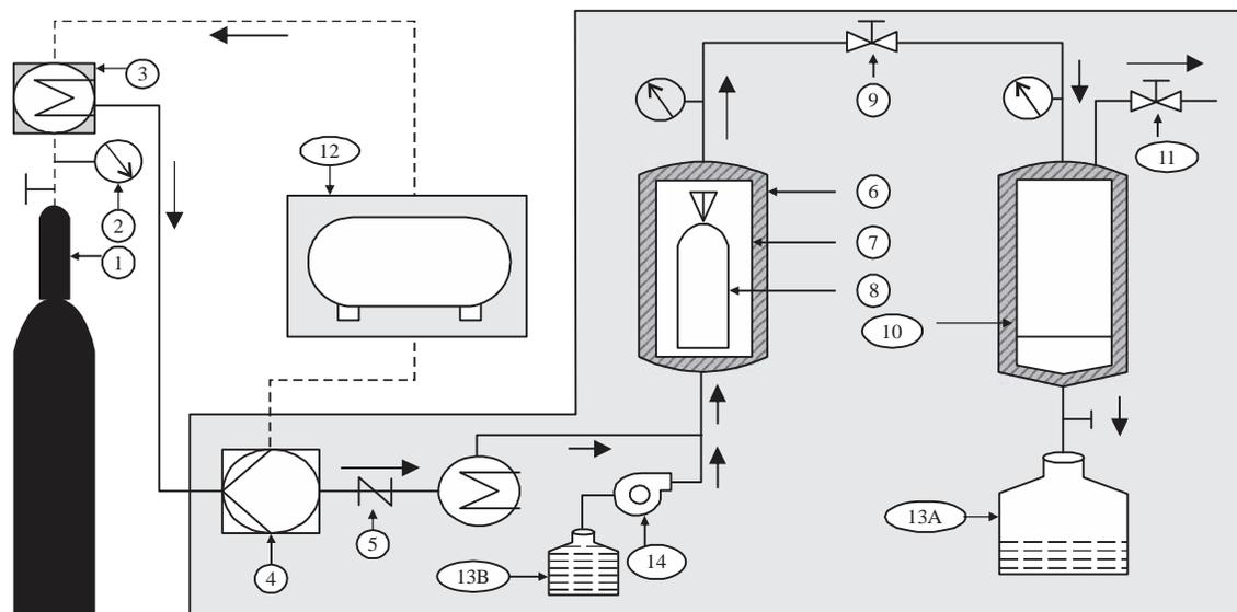
Fig. 1: Process flow chart for PLE Unit
