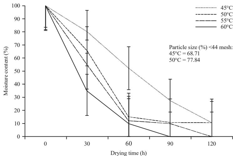
Fig. 1: Effect of drying temperature on drying of mushroom
