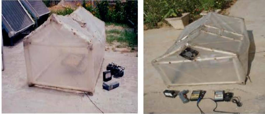
Fig. 1a, b: Experimental set-up for prawn drying inside greenhouse under forced convection mode
