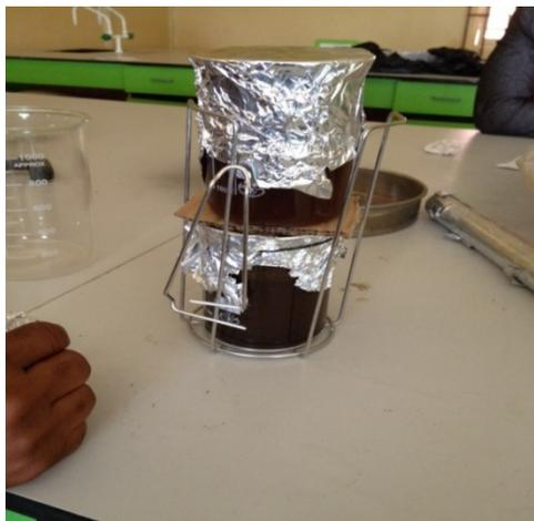
Fig. 3: Anaerobic digestion of pure liquid extract of plantain pseudostem
