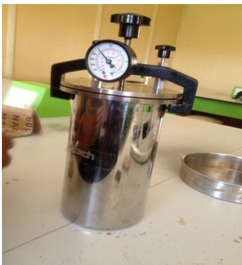
Fig. 2: Anaerobic digester containing samples undergoing co-digestion
