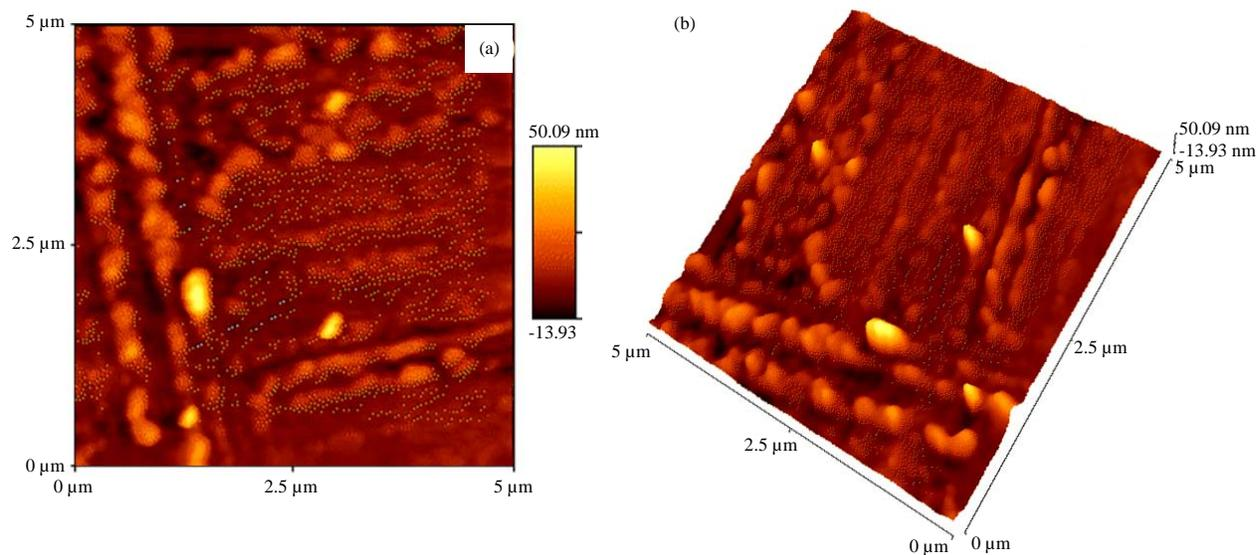
Fig. 3(a-b): AFM images of Sn doped ZnO nanoparticles (a) 2D image and (b) 3D image
