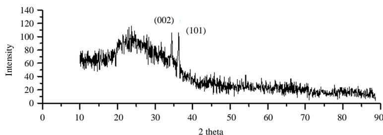
Fig. 1: XRD spectrum of Sn-ZnO nanoparticles
