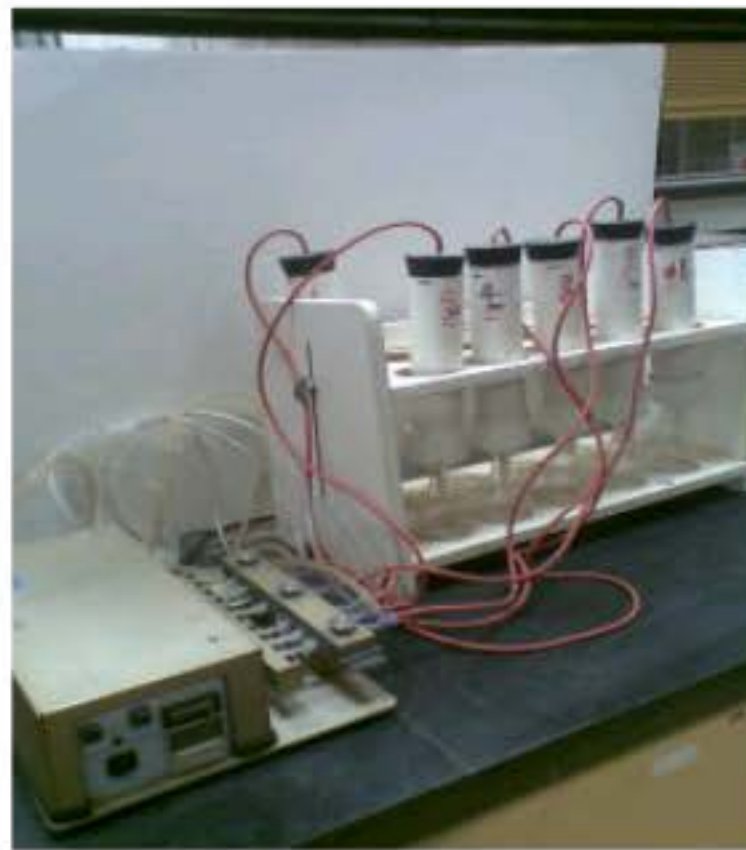
Fig. 1: A picture of the column experiment for nitrate leaching
