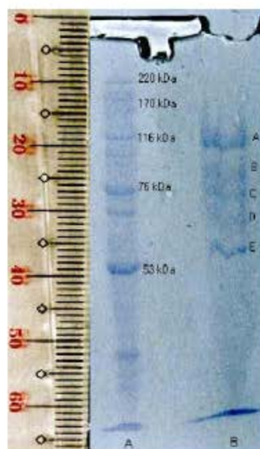
Fig. 2: SDS-PAGE of lectin from internal organs of Holothuria scabra Jaeger purified by gel chromatography. (A-MW markers, B-isolated lectin, 5 sub-units namely A=120, B=98, C=80, D=65 and E= 51 kD)
