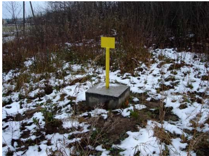
Fig. 3: Cement plinth and plate with the number of the closed borehole
