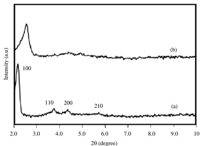
Fig. 1(a-b): Powder XRD patterns for MCM-41 samples, (a) As-synthesized MCM-41 and (b) Calcined MCM-41
