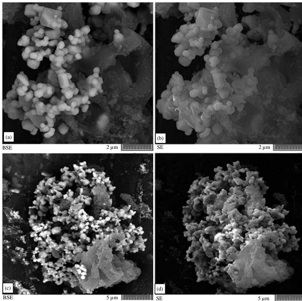
Fig. 3(a-d): Scanning electron micrographs for (a, b)  $AG_3PO_4$  and (c, d)  $AG_3PO_4/MCM-41(PS)$ .
