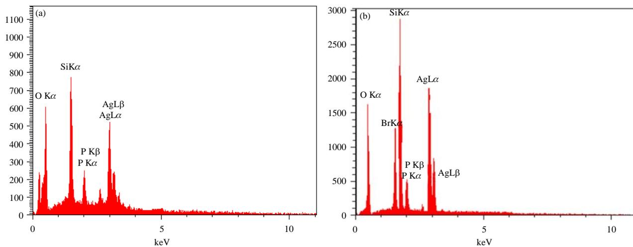
Fig. 4(a-b): EDX analysis of (a)  $AG_3PO_4/MCM-41 (PS)$  and (b)  $AG_3PO_4/MCM-41 (DS)$
