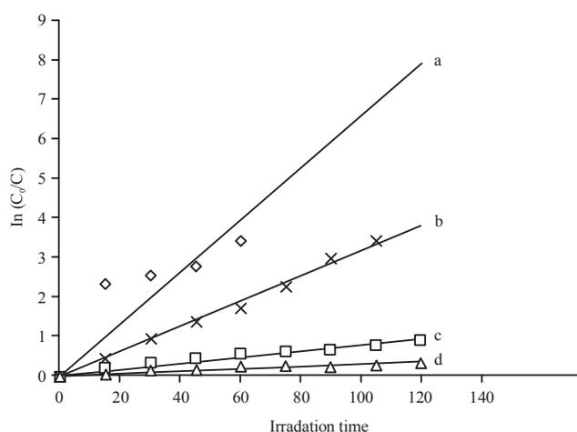
Fig. 8: Pseudo-first-order plot of (a) AG<sub>3</sub>PO<sub>4</sub>/MCM-41(PS), (b) AG<sub>3</sub>PO<sub>4</sub>, (c) AG<sub>3</sub>PO<sub>4</sub>/MCM-41(DS) and (d) MCM-41 for degradation of MB. The concentration of MB was 20 mg L<sup>-1</sup>, weight of catalyst was 50 mg and volume of dye solution 50 mL, photocatalytic reaction under visible light irradiation at room temperature and the system was open to air
