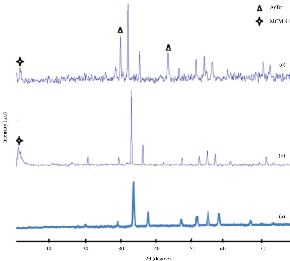
Fig. 2(a-c): Powder XRD patterns for, (a)  $AG_3PO_4$ , (b)  $AG_3PO_4/MCM-41(PS)$  and (c)  $AG_3PO_4/MCM-41(DS)$
