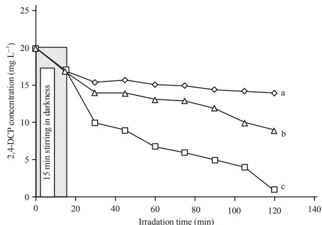
Fig. 7: Concentration changes of 2,4-DCP as a function of time using  $\text{AG}_3\text{PO}_4/\text{MCM-41}(\text{PS})$  in various conditions, (a) Dark, (b) Irradiated by visible light and (c) Irradiated by UV-A light. The initial concentration of 2,4-DCP was  $20 \text{ mg L}^{-1}$ , weight of catalyst was  $40 \text{ mg}$ , volume of the dye solution  $50 \text{ mL}$
