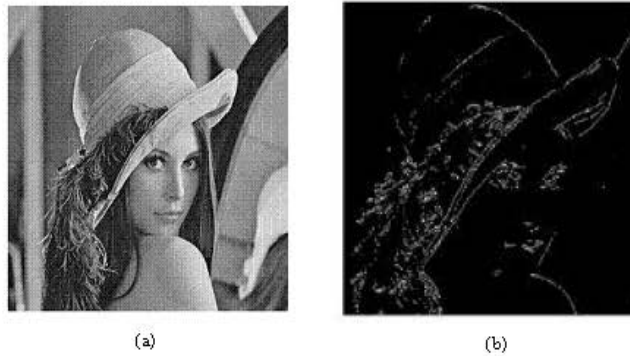
Fig. 6: (a) Original Lena Image and (b) After averaging and edge detection templates by employing RK-heronian mean algorithm
