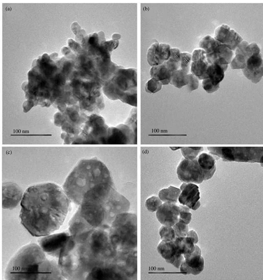
Fig. 3(a-b): TEM images for (a) ZnO, (b) 0.01M SnO<sub>2</sub> doped ZnO, (c) 0.04 M SnO<sub>2</sub>/ZnO and (d) 0.05 M SnO<sub>2</sub>/ZnO
