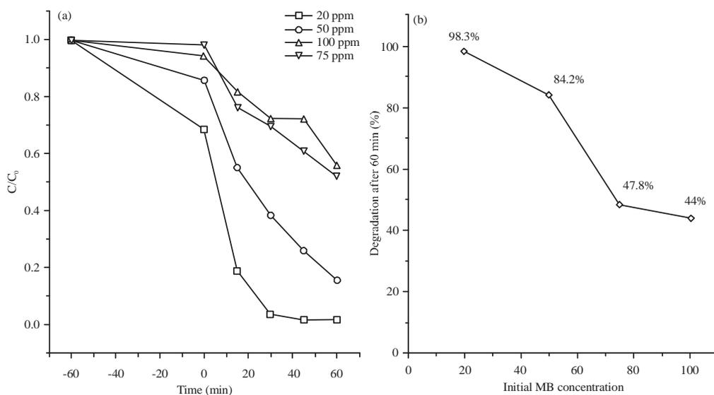
Fig. 5(a-b): (a) Effect of initial concentration of methylene blue on the photodegradation efficiency of 0.04 SnO<sub>2</sub>/ZnO, (b) Degradation for methylene blue after 60 min at pH 10 over 0.04 M SnO<sub>2</sub>/ZnO
