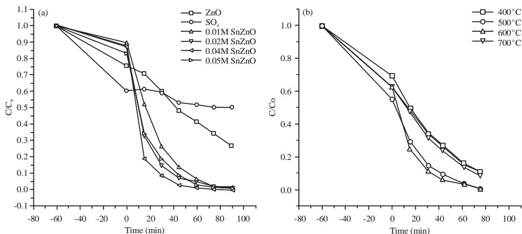
Fig. 4(a-b): Photodegradation curves of methylene blue on (a) ZnO, SnO<sub>2</sub> and SnO<sub>2</sub> doped ZnO and (b) 0.04 M SnO<sub>2</sub>/ZnO, treated under different temperatures
