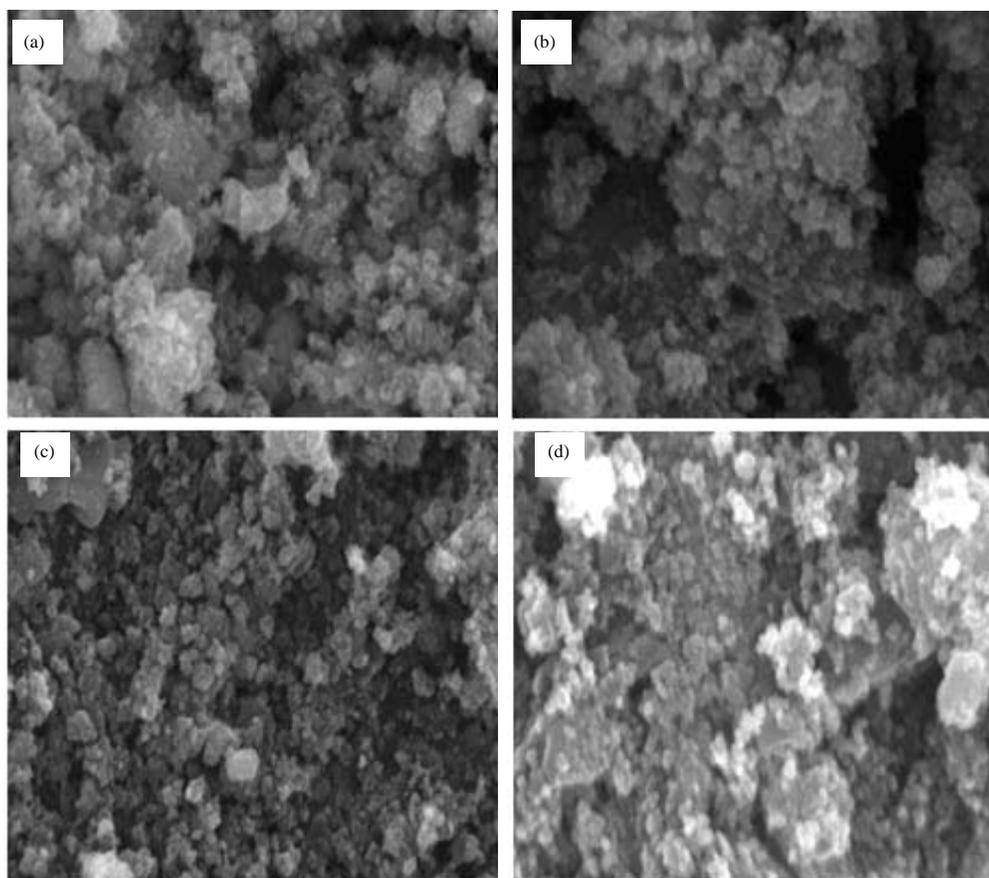
Fig. 2(a-b): SEM images for (a) ZnO, (b) 0.01 M SnO<sub>2</sub>/ZnO, (c) 0.04 M SnO<sub>2</sub>/ZnO and (d) 0.05 M SnO<sub>2</sub>/ZnO
