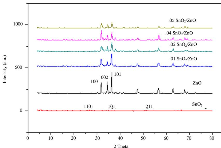
Fig. 1: XRD pattern for ZnO and SnO<sub>2</sub> doped ZnO calcined at 600°C
