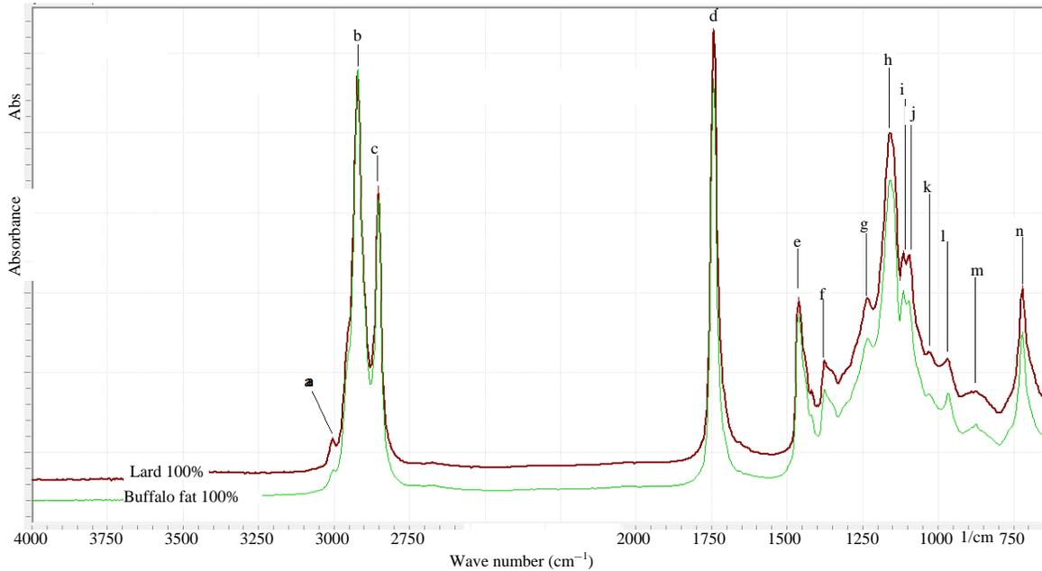
Fig. 1: FTIR spectra of lipid fraction extracted from Rambak cracker containing 100% buffalo skin (buffalo fat) and 100% pig skin (lard) at mid infrared region (4,000-650  $\text{cm}^{-1}$ )
