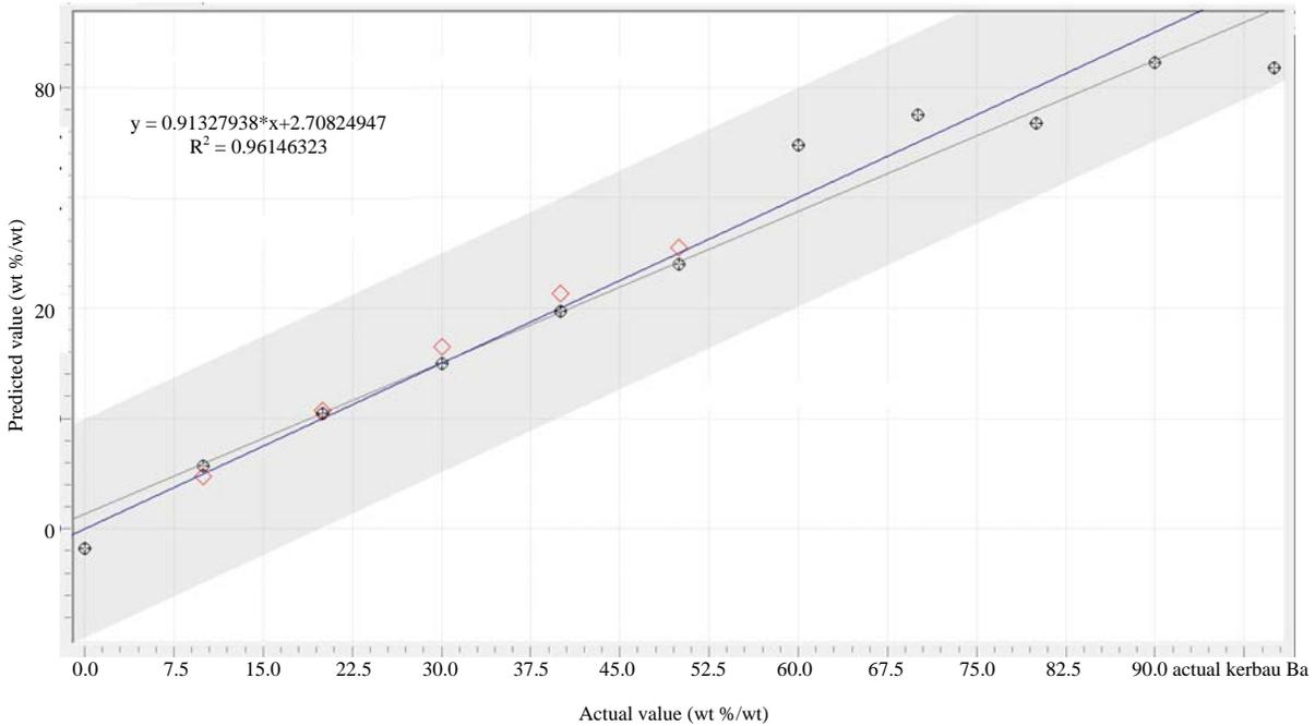
Fig. 4: Calibration model of PLS for the relationship between actual and FTIR predicted value of buffalo fat adulterated with lard using spectra  $1200-1000\text{ cm}^{-1}$
