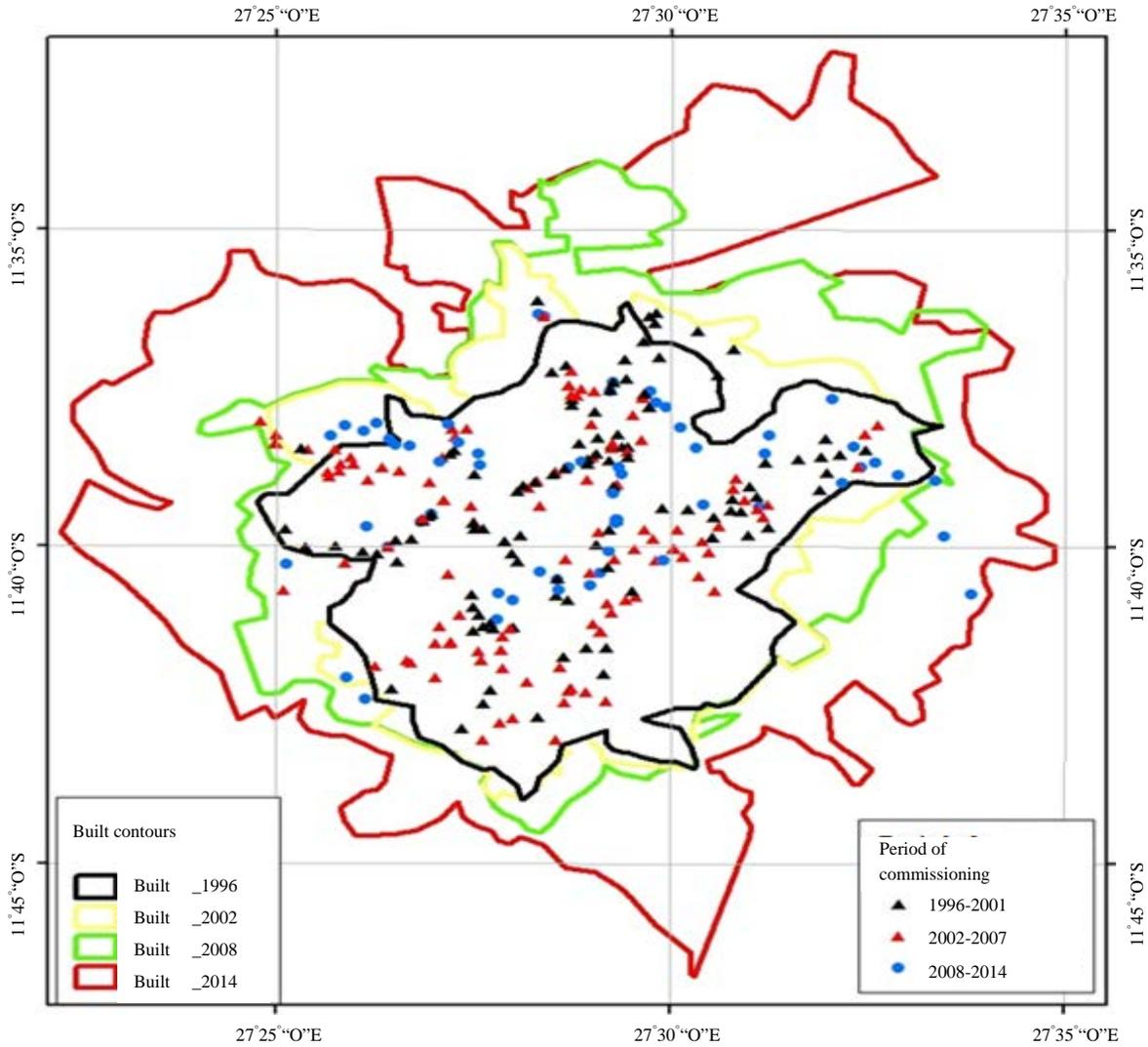
Fig. 3: Temporal distribution of electric cabins in Lubumbashi. Information on the commissioning date of each electrical cabin were found in the database of the National Electricity Company (SNEL). For SNEL and private cabins, information was obtained through terrain survey that allowed to interview the inhabitants of neighborhoods
