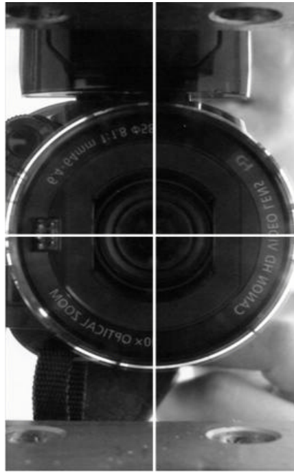
Fig. 2: Mirror image used to detect out-of-plane displacement
