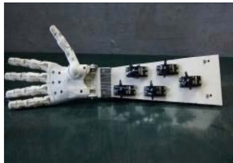
Fig. 13: Robotic fingers connected with servo motors
