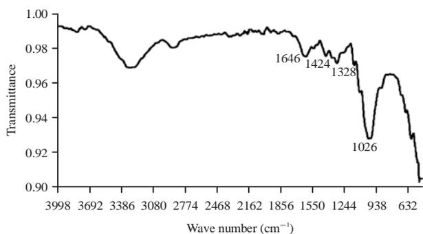
Fig. 8: FTIR spectrum of ramie fibre
