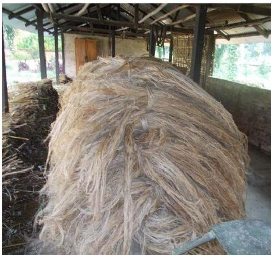
Fig. 5: Decorticated fibre
