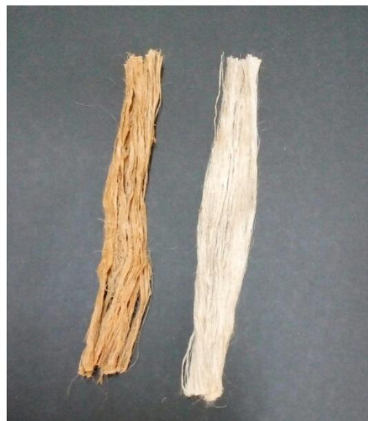
Fig. 7: Decorticated and degummed ramie fibre
