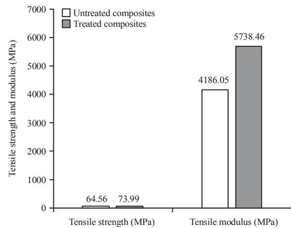
Fig. 3: Tensile strength and modulus of composites
