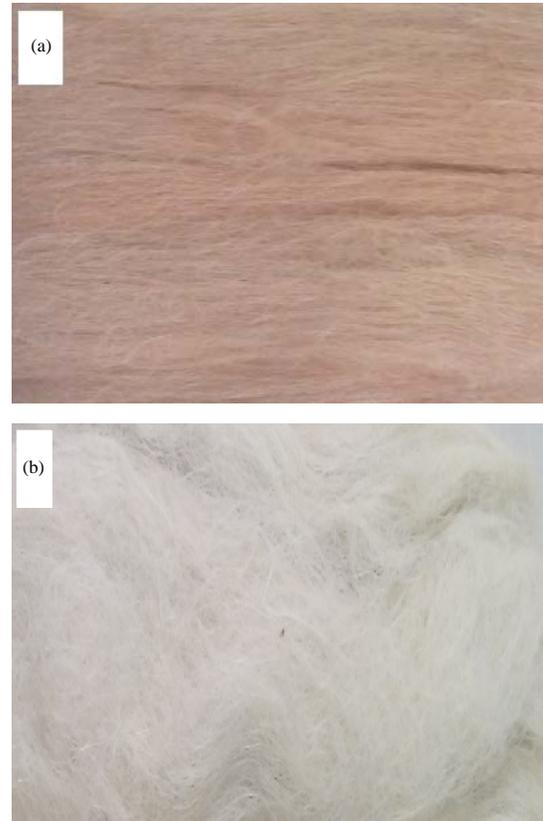
Fig. 2(a-b): Jute fibres (a) Untreated and (b) Treated
