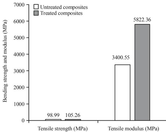
Fig. 5: Bending strength and modulus of composites
