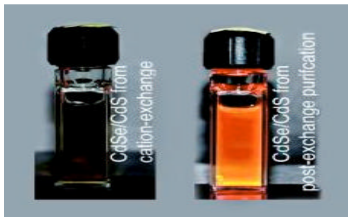
Fig. 5: Luminescence of CdSe/CuS nanocrystals prepared by cation-exchange. Left picture showing crystals before purification and the right picture are the same nanocrystals after purification in which impurities have been removed. (Credit: Image courtesy of DOE/Lawrence Berkeley National Laboratory)
