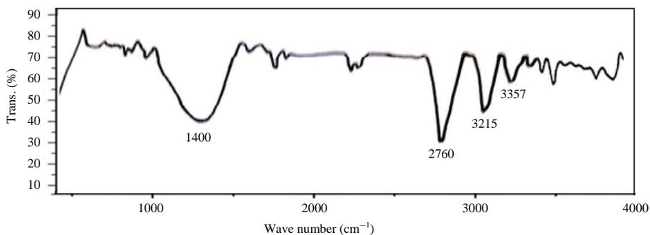
Fig. 5: FTIR spectra of pure zein polymer
