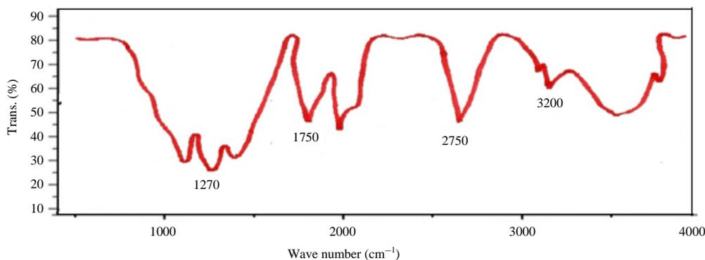
Fig. 4: FTIR spectra of uncoated ZnO nanoparticles
