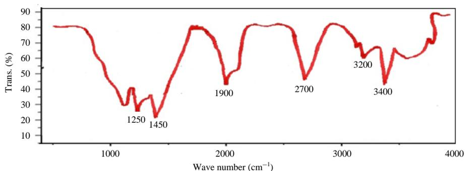
Fig. 6: FTIR spectra of zein coated ZnO nanoparticles
