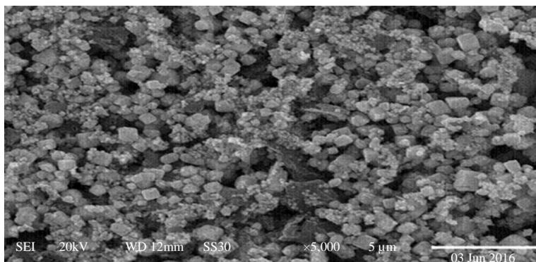
Fig. 2: Scanning electron microscope (SEM) of Ag nanoparticles
