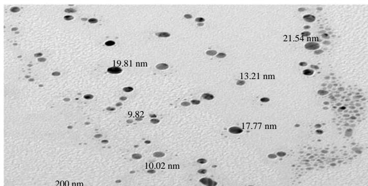
Fig. 3: Transmission electron microscopic image of silver nanoparticles biosynthesized by *Ulva fasciata* aqueous extract and stabilized by SDS
