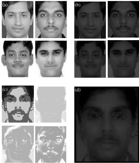
Fig. 4(a-d): Images of cropped faces (a) Training set, (b) Normalized training set, (c) Eigenfaces and (d) Mean image
