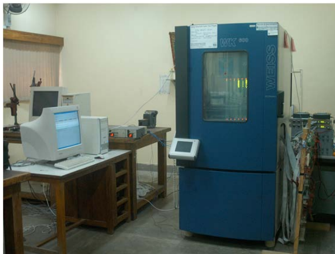
Fig. 8: Typical test setup for environmental testing of embedded system
