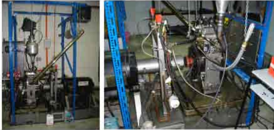
Fig. 17: The SCRE test rig of CNG-DI engine
