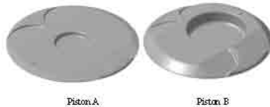
Fig. 2: Geometry of the combustion chamber
