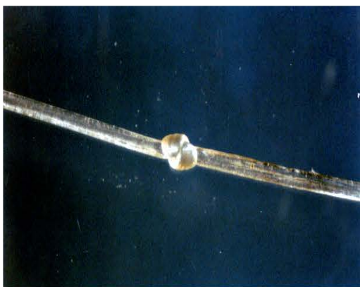
Fig. 6: Knot ability of GT fiber with the aid of glycerin
