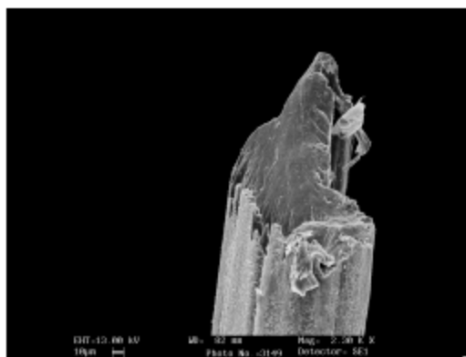
Fig. 4: Forming of sheet core structure due to high concentration of coagulant agent ( \text{CaCl}_2 as coagulant agent with 150 \text{ g L}^{-1} concentration)
