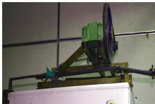
Fig. 1: Freezer cabinet automatic door opening mechanism
