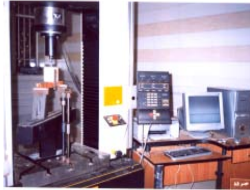
Fig. 2: Static bending test assembly
