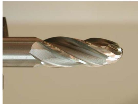
Fig. 10: The actual produced ball-end taper milling cutter
