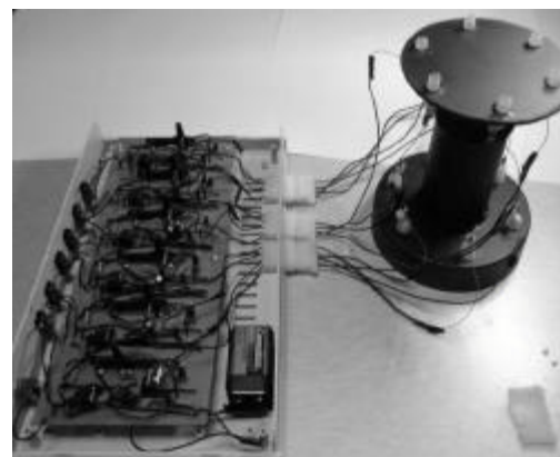
Fig. 13: Stewart platform and PWM control box
