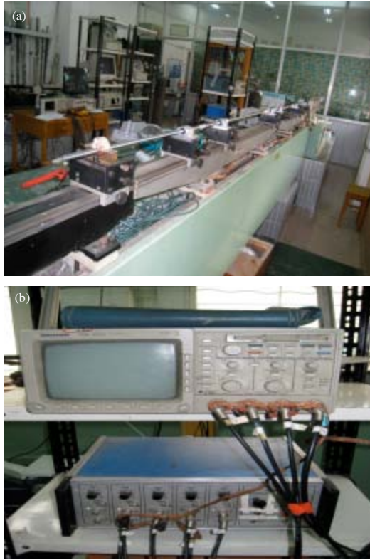
Fig. 4(a-b): Experimental equipment for Split Hopkinson Pressure Bar to obtain material data
