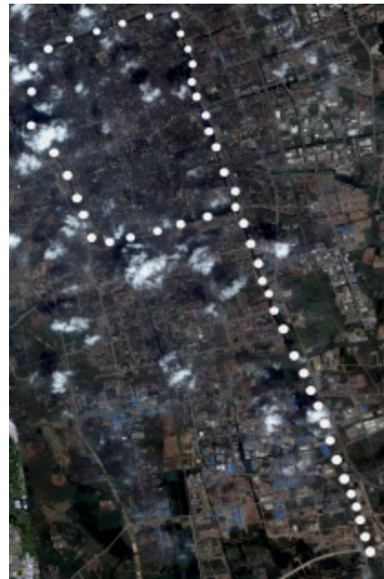
Fig. 1: Map of sampling position of the river network areas in the SuZhou city, china. Spectra, Total Phosphorous (TP), Total Nitrogen (TN) sampled in stations including 50 locations were measured and analyzed and K, Mg and Cu were sampled in 10 of all locations, on December 23 in 2009
