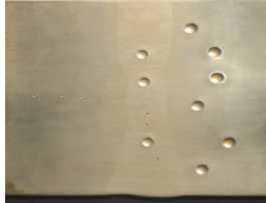
Fig. 6: Weld specimen hardness measuring icon (100 mm)
