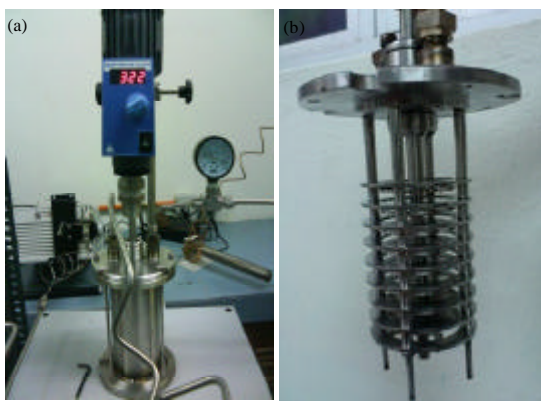
Fig. 1(a-b): (a) Rotating disc contactor (RDC) column and (b) Rotating disc
