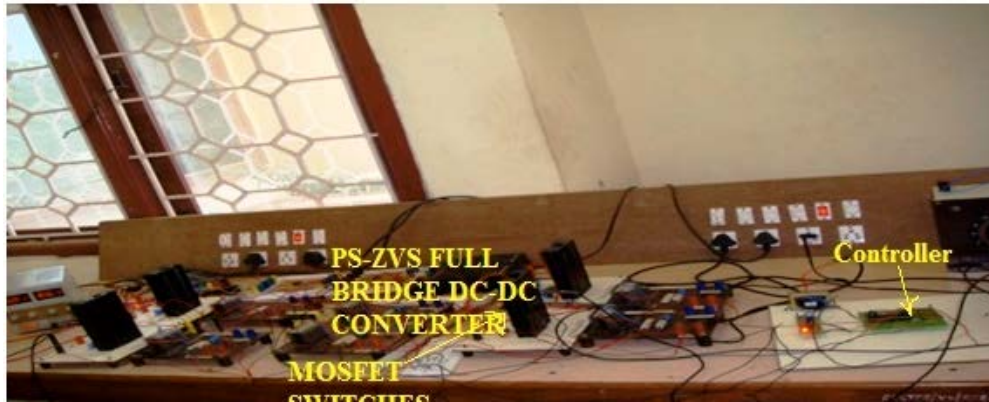
Fig. 7: Experimental setup of the PS-ZVS full bridge dc-dc converter
