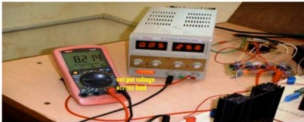
Fig. 8: Load voltage of full bride Dc-Dc converter
