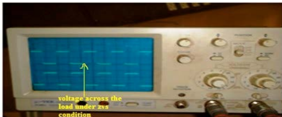
Fig. 9: Voltage across the load under zero voltage switching condition
