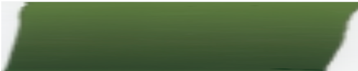
Fig. 7: A strip of Gafchromic EBT2 film (20×3 cm 2 ) irradiated to 500 MU from 6 MV photon beam parallel with the central beam axis
