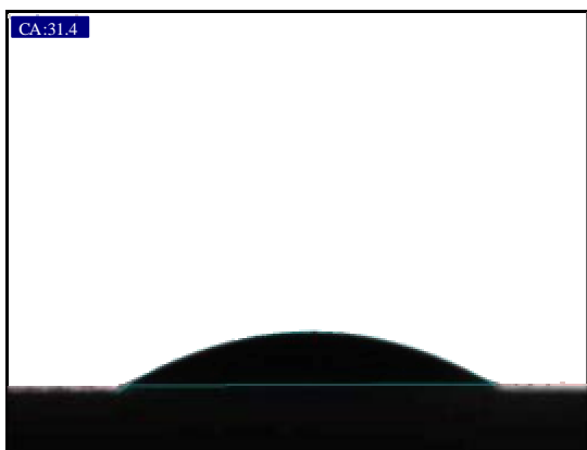
Fig. 3: Sessile drop images for the 50:15:4.5 ratio
