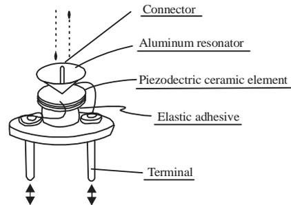
Fig. 2: Topology of ceramic-film ultrasonic transduce
