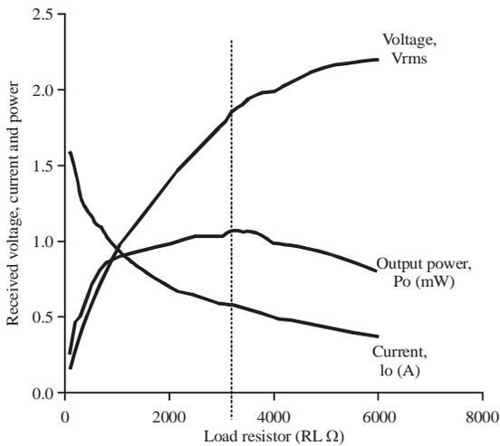
Fig. 7: Optimal power transfer ratio increases with an increase in load resistance. The most optimum value is at 3.3 kΩ load resistances where 1.071 mW power is obtained
