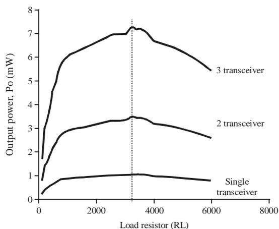
Fig. 11: Result of multiple input-output AET system. The maximum power of the system is 1.07 mW for single transceiver, 3.47 mW for two transceivers and 7.24 mW for three transceivers
