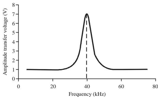
Fig. 4: Amplitude vs frequency of the AET initial experiment
