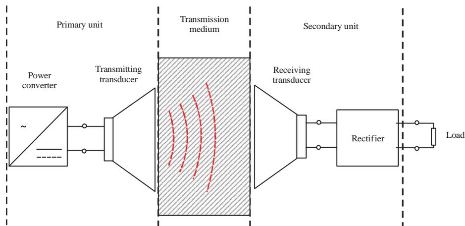
Fig. 1: A typical AET system that consists of 3 parts; primary unit, transmission medium and secondary unit
