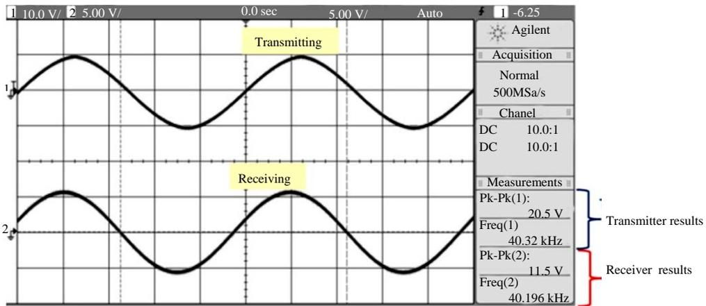
Fig. 3: Result of transmitting voltage from function generator
