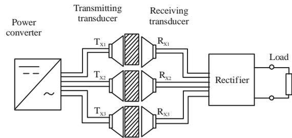
Fig. 9: Multiple input-output AET system block diagram
