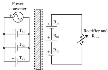
Fig. 10: Connection of multiple transmitters,  $T_x$  in parallel and multiple receivers,  $R_x$  in series
