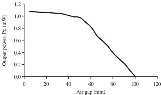
Fig. 8: AET system with different air gap between transducers input-output of the transducer is used. The arrangement of the system is shown as in Fig. 9. The ultrasonic
