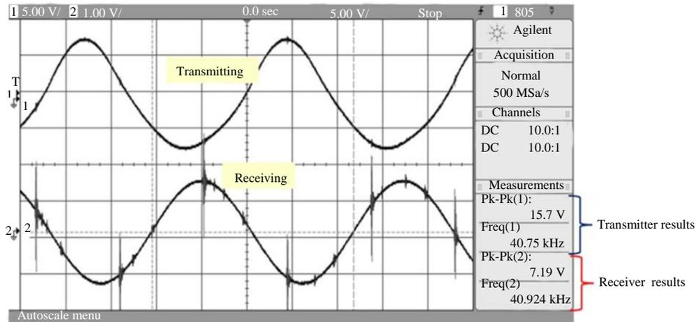
Fig. 6: Result of push-pull power converter on AET
