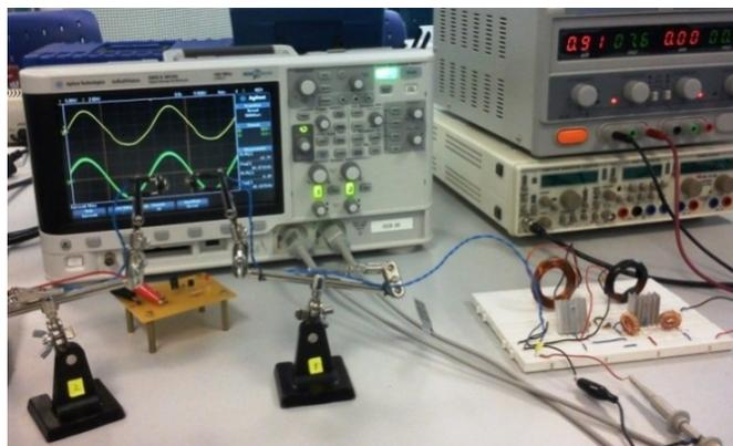
Fig. 5: AET system experimental setup shows AET basic system using push-pull power converter transmits energy through the air medium
