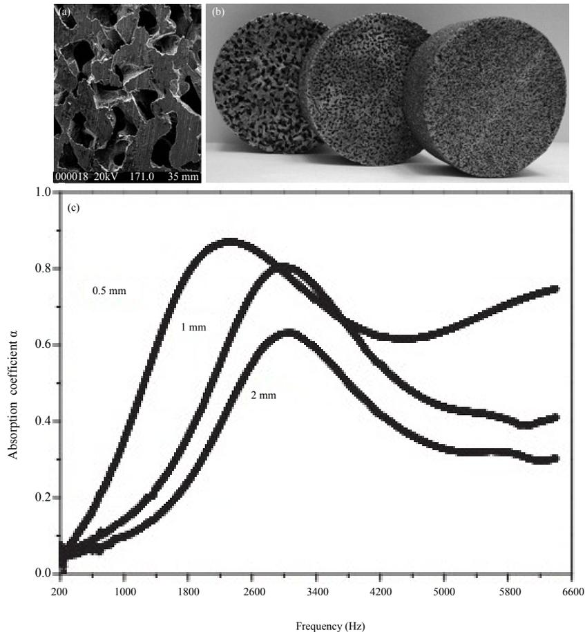
Fig. 4(a-c): (a) SEM image of the interconnected pores in AISiMg alloy/NaCl composite<sup>76-85</sup>, (b) Different samples with different pore size prepared by infiltration process<sup>76-85</sup> and (c) Dependence of pore size of the sample on the sound absorption coefficient<sup>76-85</sup>
