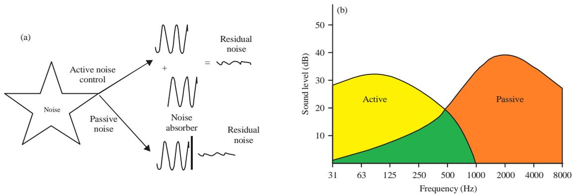
Fig.1(a-b): (a) Active and passive noise control mechanisms<sup>9</sup>, (b) Frequency response region of the active and passive noise control methods<sup>9</sup>
