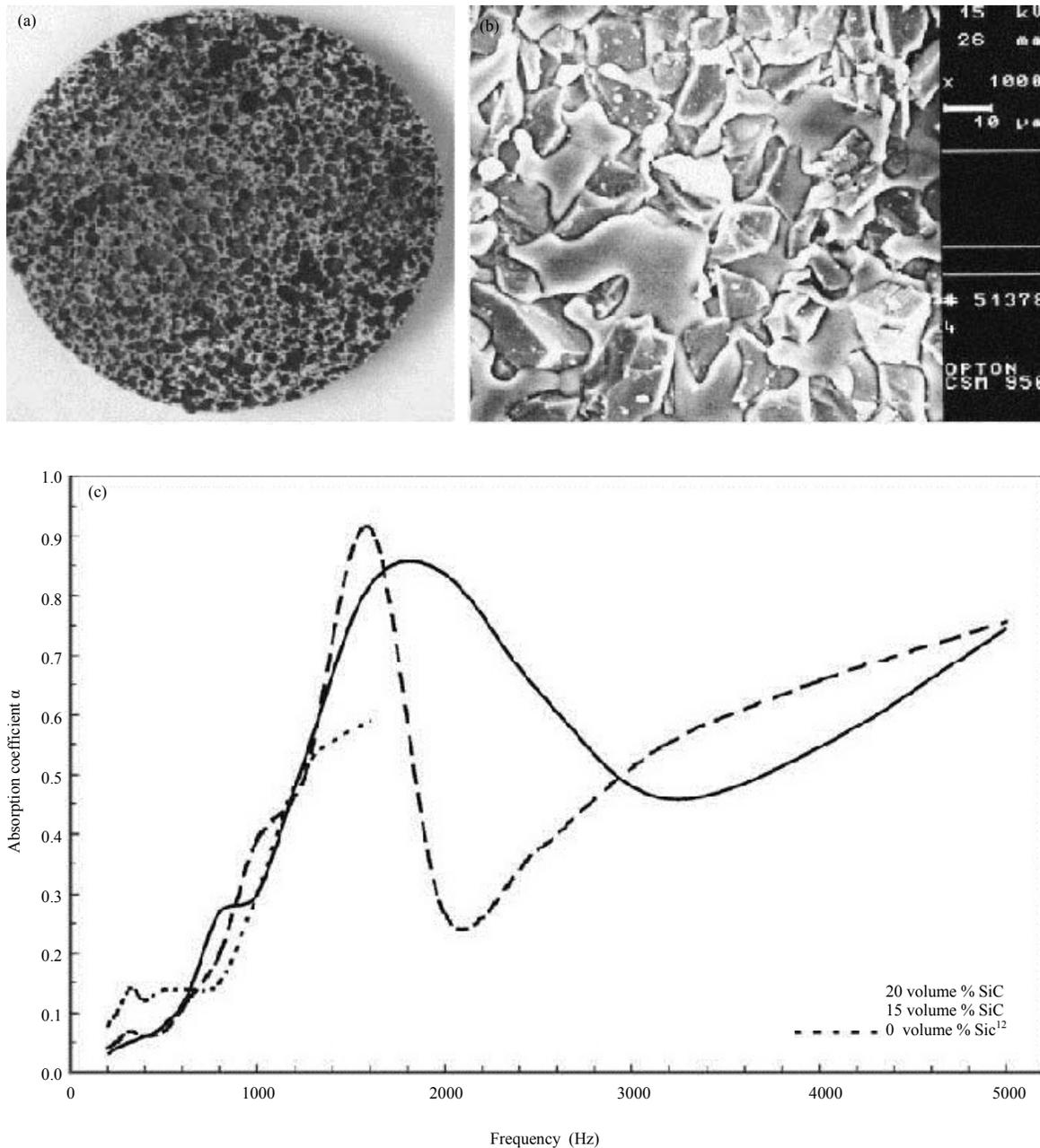
Fig. 5(a-c): (a) Typical macro graphic structure of A356/20SiCp composite foams<sup>82</sup>, (b) SEM image of cell surface of A356/20SiCp composite foams<sup>82</sup> and (c) Influence of frequency and SiCp content on sound absorption coefficient<sup>82</sup>
