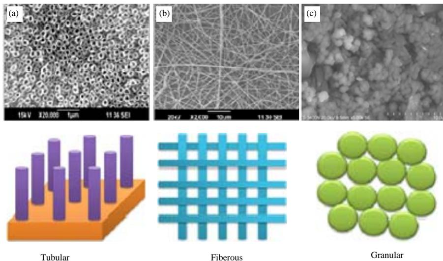
Fig. 2(a-c): Scanning electron microscope images and schematic representation of porous absorbers, (a) Tubular structure, (b) Fibrous structure and (c) Granular structure
