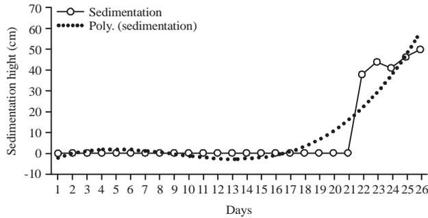
Fig. 3: Sedimentation of sludge in the UASB digester design research
