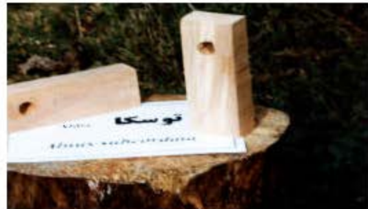
Fig. 2: Alder samples after drilling
