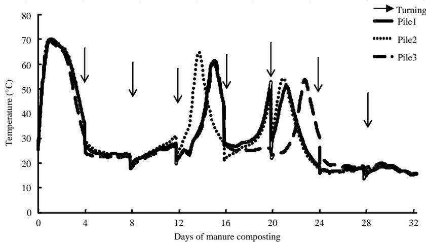
Fig. 2: Changes in temperature of poultry composted mixture during the first 32 days after composting in the main experiment
