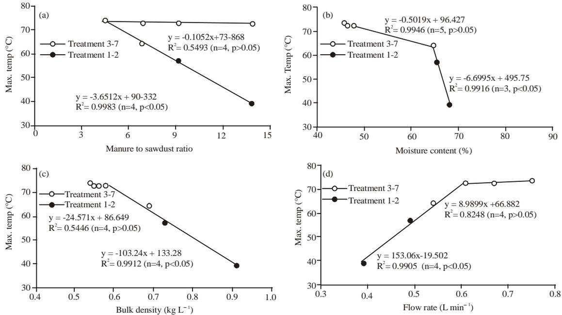
Fig. 1(a-d): Relationships between (a) Manure-to-sawdust ratio, (b) Moisture content of composted mixture, (c) Bulk density of the composted mixture and (d) Flow rate and the maximum temperature (Max temp) of the mixture during the first 7 days after composting in the preliminary experiment
