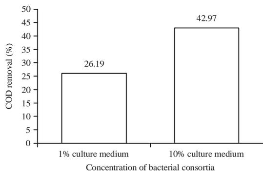
Fig. 3: Effect of concentrations of bacterial consortia in culture medium on COD removal in tempeh wastewater
