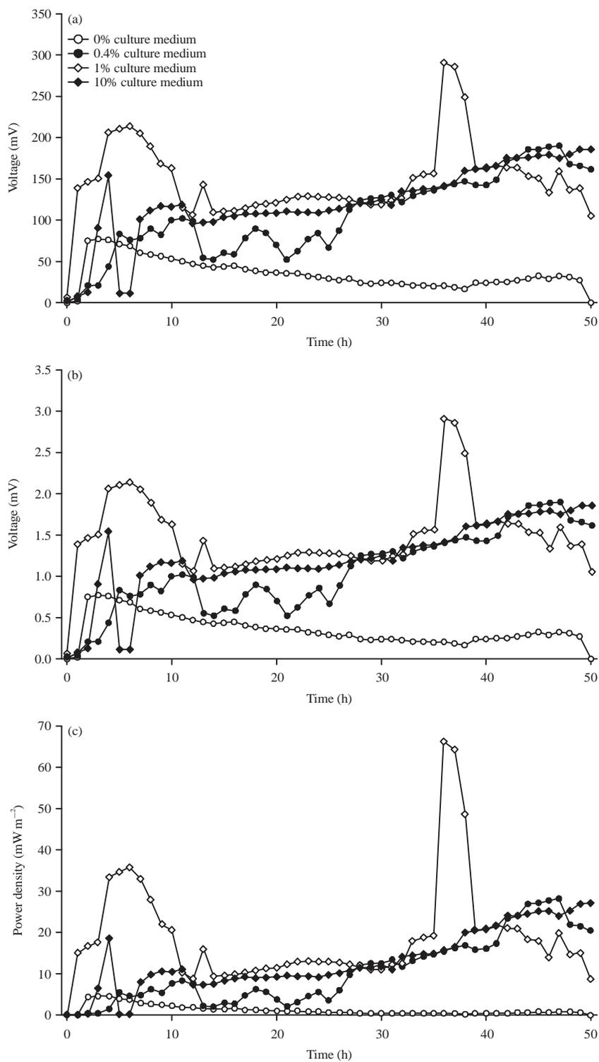
Fig. 1(a-c): Effect of 0, 0.4 and 1% dan 10% of bacterial consortia in culture medium on (a) Voltage, (b) Current and (c) Power density
