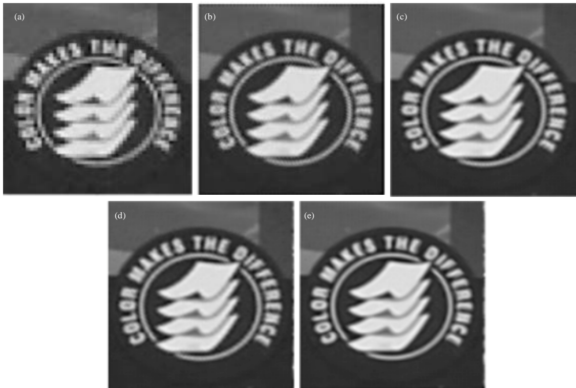
Fig. 7(a-e): An example of HR reconstruction from different super resolution methods; Results (2x resolution increase) by (a) Original low resolution image interpolated by nearest neighbor interpolation, (b) Tikhonov regularization, (c) Variational Bayesian SR, (d) Total-variation regularization SR and (e) Proposed method
