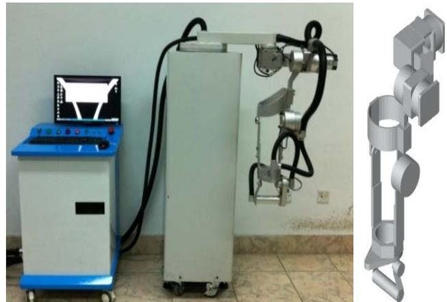
Fig. 1: Training system of the 5 DOF exoskeleton robot for upper limb rehabilitation
