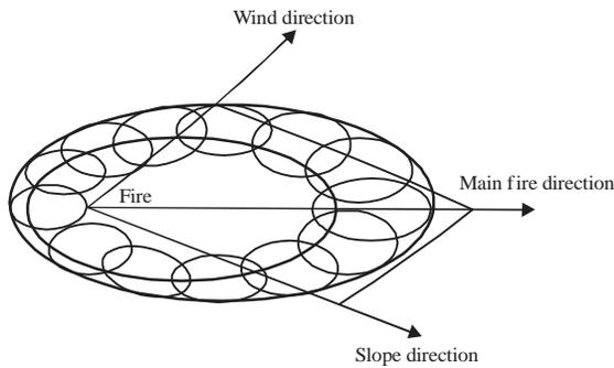
Fig. 3: Calculation and simulation method based on Huygens principle
