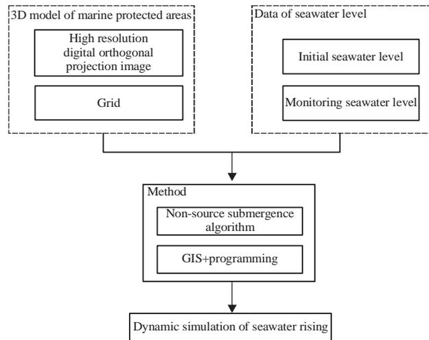
Fig. 4: Simulation process of seawater rising
