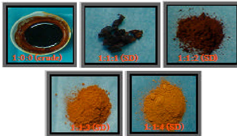
Fig. 1: Characteristic of mixture sample from the ratios of TO, PEG400 and MgO by solid dispersion (SD)
