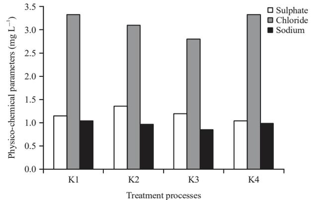
Fig. 3: Effect of Kent water treatment processes on sulphate, chloride and sodium
