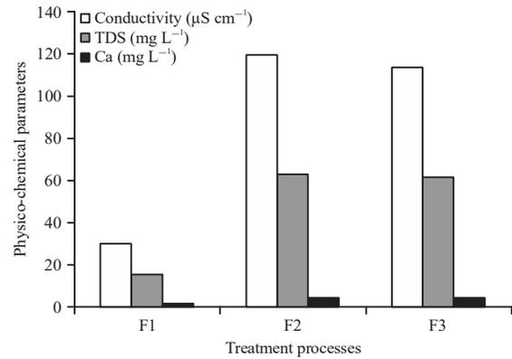
**Fig. 8:** Effect of Fressi water treatment processes on conductivity, TDS and calcium
