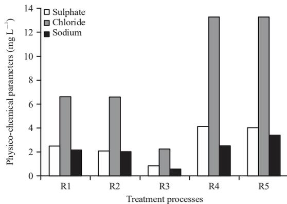
**Fig. 6:** Effect of Rivoli water treatment processes on sulphate, chloride and sodium
