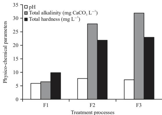
**Fig. 7:** Effect of Fressi water treatment processes on pH, total alkalinity and total hardness
