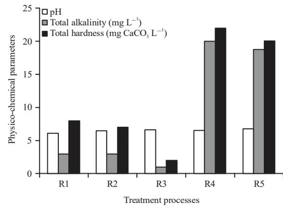
Fig. 4: Effect of Rivoli water treatment processes on pH, total alkalinity and total hardness
