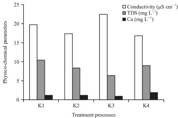
Fig. 2: Effect of Kent water treatment processes on conductivity, TDS and calcium
