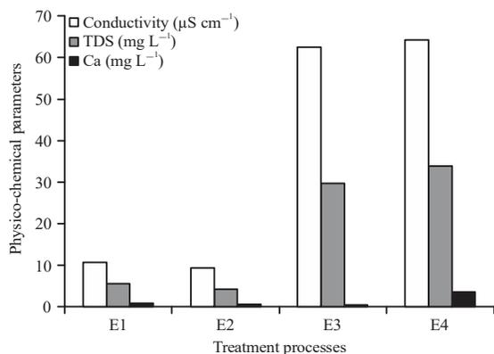
Fig. 11: Effect of Elioaha water treatment processes on conductivity, TDS and calcium
