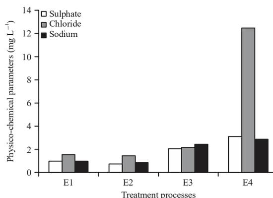
Fig. 12: Effect of Elioaha water treatment processes on sulphate, chloride and sodium
