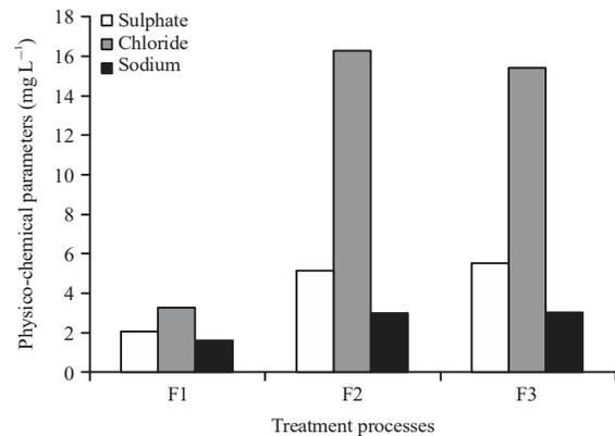
**Fig. 9:** Effect of Fressi water treatment processes on sulphate, chloride and sodium
