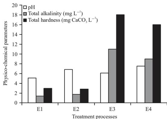
Fig. 10: Effect of Elioaha water treatment processes on pH, alkalinity and total hardness
