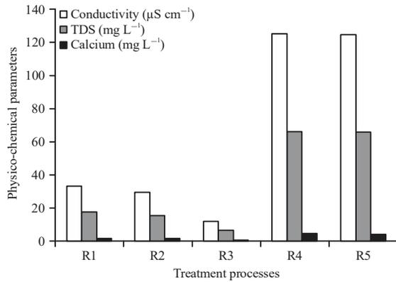
**Fig. 5:** Effect of Rivoli water treatment processes on conductivity, total dissolved solids and calcium
