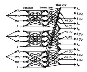
Fig. 1: Neural network for 3D motion estimation
