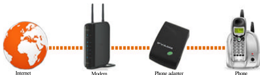
Fig. 1: ATA device, standard Phone and Internet
