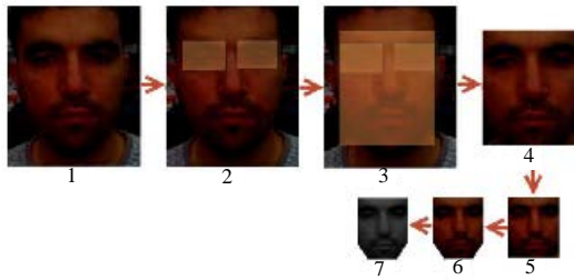
Fig. 17: Isolate the face area based on the eyes location example, then Apply special mask to isolate the face area well
