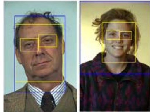
Fig. 12: Hybrid algorithm implementation examples, the result of detection based on skin color (blue rectangle), the result of detection based on Viola-Jones (yellow rectangles)
